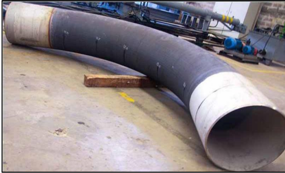
Induction bends (bending through heating)
